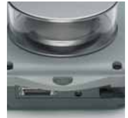
RS-232 data interface and anti-theft locking device
